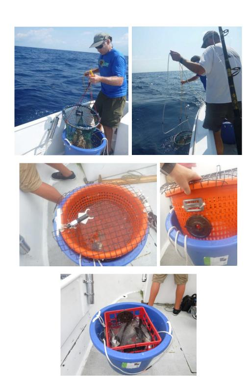
**Figure 6.**Multi-fish descending devices trialed offshore of Hatteras, N.C., July 2015 in a supplemental trial. The top left photo shows the l8-inch net, being prepared for deployment over the rail of the ("6 pack") boat. The top right photo features the net being lowered into the water; the middle left photo displays the crab basket with the wire trap door and Seaqualizer closure. The middle right photo shows the weights (10-pounds) attached to the basket. The bottom photo illustrates
