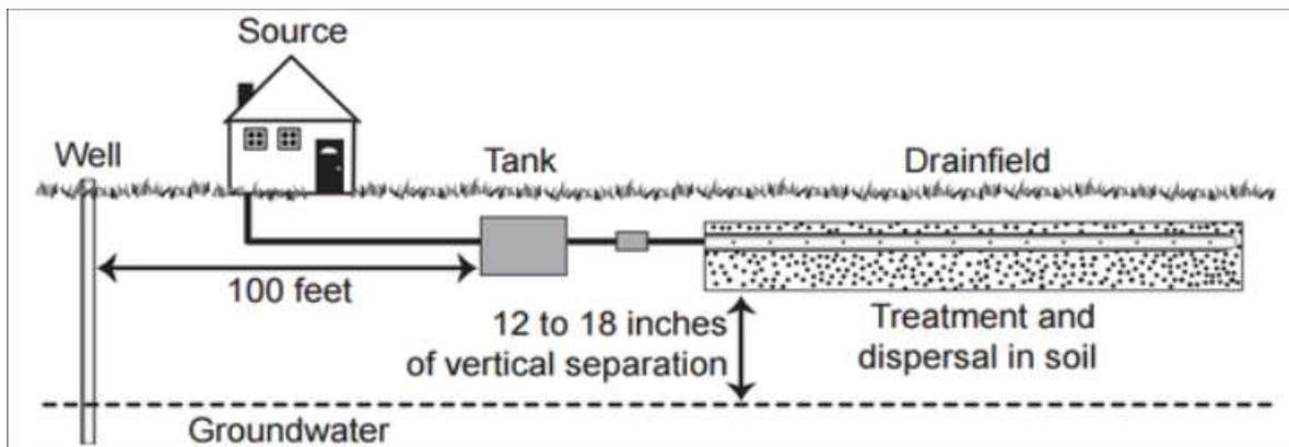
**Figure 2.1.** Vertical separation distance requirements for conventional systems in North Carolina.<sup>27</sup>
