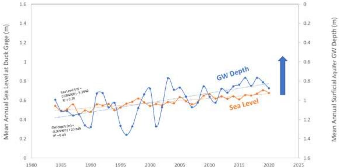
**Figure 3.8.** Comparison of mean annual sea level at the NOAA Duck, NC tidal gage and mean annual groundwater depth in NC DEQ surficial aquifer wells (8 sites) in Dare County, NC. Note that the groundwater depth axis is inverted (0=land surface and greater depths are to the bottom of the figure). Data sources: NOAA and NC DEQ.
