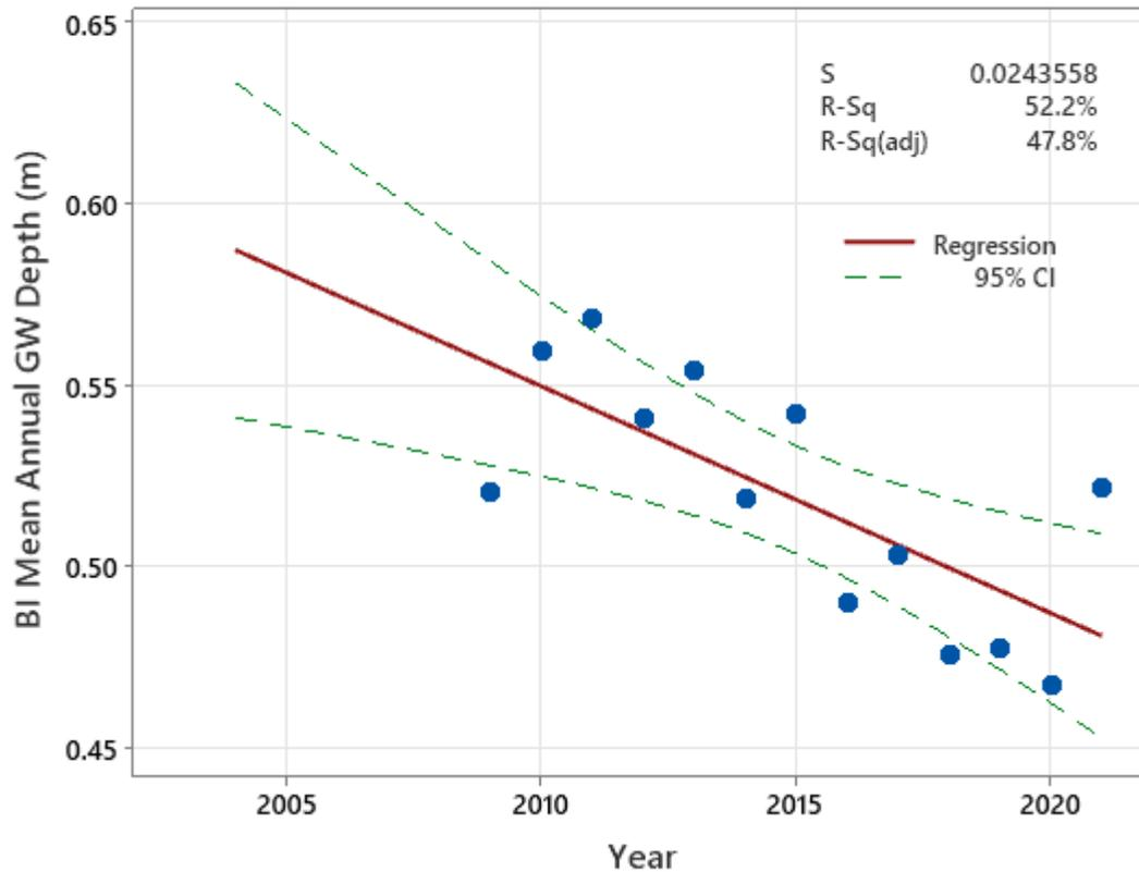
**Figure 3.10.** Mean annual groundwater depths measured in the surficial aquifer at Bodie Island (BI) based on daily data since 2008 collected by NC DEQ. The trend suggests a 6.3 mm/yr groundwater rise in this area from 2008-2021.
