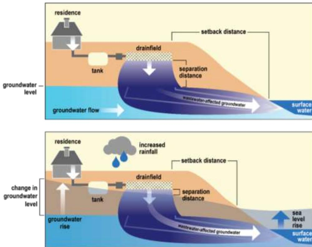
**Figure 2.2.** How rising sea levels, groundwater levels and increased rainfall reduce the separation distance needed for onsite wastewater treatment. Source: Illustration by Melissa D. Smith<sup>34</sup>
